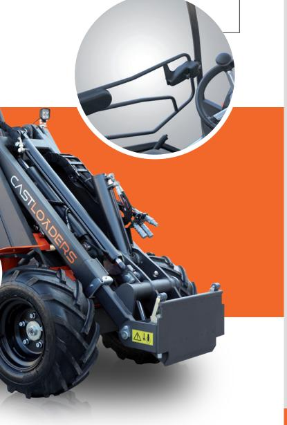
Cast 820D is equipped with a Kubota D722 diesel engine, liquid cooled, 4WD hydrostatic transmission and 10km / h speed. Electric differential lock, 5-function joystick, silent block, tractor tires 23x8.50-12.
