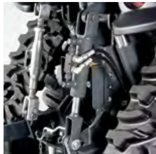
VERTICAL TIE-ROD Optimises the positioning and inclination of the equipment.
