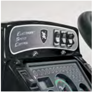
ESC (Electronic Speed Control) Electronic and automatic speed and engine rev control device.
