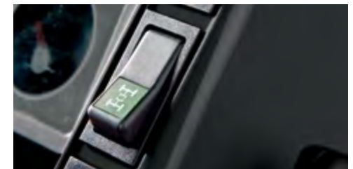
The rear differential lock prevents slipping and optimises traction. The front traction disengagement is useful when travelling along roads and prevents damage from being done to delicate grounds.
