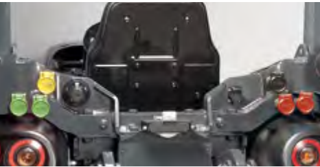
Hydraulic system with 2 double-acting manifolds, 1 single-acting + oil return tap.
