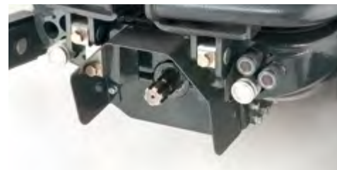
The front PTO* (1000 rpm) with electrohydraulic controls and progressive engagement with safety button is maintenance free.
