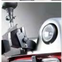
Front and rear working lights assembled in the cab roof and foldable number plate holder.
