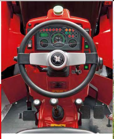
Thanks to the ACTIO™ Chassis, the driving position coincides with the center of oscillation of the tractor. Sideways jerking and stress are very limited and operator fatigue is reduced, even after many hours. The on-board instrumentation is elegant, functional and intuitive: backlit anti-reflection screen for nighttime use; "on-off" information system; digital tachometer and PTO rev counter; and electro-hydraulic pushbutton controls.
