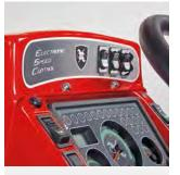
ESC (Electronic Speed Control) Electronic and automatic speed and engine rev control device. It memorises and modulates the tractor speed at the operator's discretion (only for the model 7800).
