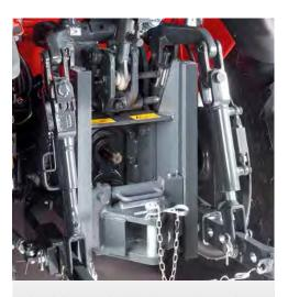
The slider\* tow hook with rapid vertical adjustment, is used to optimize the connection height of the towed equipment.
