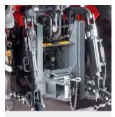
**SLIDER HOOK**Integrated into the rear lift, it gives the operator various options for the practical setting up of the tractor and the rapid alignment of the towed equipment.
