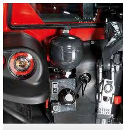
Hydropneumatic suspension with automatic pressure control.
