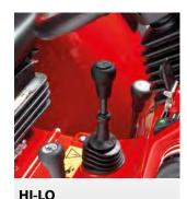
HI-LO system which can be electro-hydraulically engaged when loaded thus reducing set speeds by 20% (64 speeds, 32 forward and 32 reverse).
