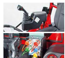
Hydraulic system with electro-hydraulic control with joystick: 2 double-acting manifolds, 1 single-acting, 1 oil return tap. Total: 6 rear quick-couplers.
