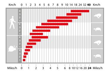
The tractors in the Ergit 100 series utilize large, extraordinarily reliable, smooth engaging clutches that do not require adjustment thanks to the hydraulic control, which recovers the play caused by wear over time. The gear has a helical profile: 32 speeds, 16 FW and 16 RV, with a synchronized inverter that can be engaged even when the tractor is moving. The small gap between one gear and the next assures operative continuity in all circumstances.
