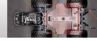
**ACTIO™**, This Full Chassis with Oscillation is comprised of a solid cast-iron chassis fixed to the axles and housing the tractor transmission. It features a central joint with a longitudinal oscillation of up to 15°. The two oscillating ends follow the contour of the terrain independently, thus assuring stability and traction at all times. The constant adherence of the tires to the ground allows engine power to be entirely transferred to the ground, thus increasing performance and safety.
