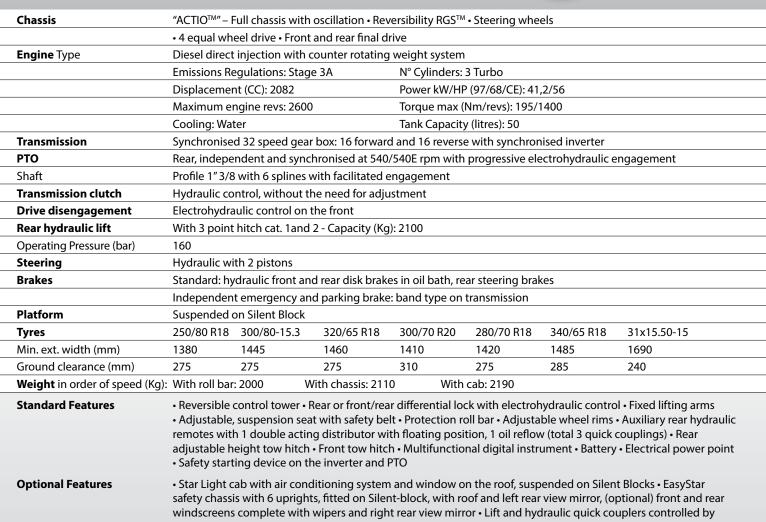
double speed "ON/OFF" Joystick • Rear power lift with suspension (2+2 pistons) • Hydraulic power lift with draft and position control • Front power lift • Hydraulic third hitch and vertical tie-rod • Adjustable lifting arms with quick release couplings • Pneumatic seat • Slider tow hitch • Pair of front/rear ballasts • Cast iron wheel flanges for 20" rear wheels • Front bullbar
