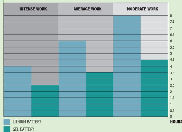
Cast 800 ECO is available with two different types of traction batteries. Gel battery: 48 Volt / 210 Ah, gel technology, sealed and maintenance free with improved safety, free from liquid leaks. Lithium battery: 48 Volt / 210Ah, longer life charge even in conditions of intense work, lower weight and higher life cycle. The charging times for both types of battery can vary from a minimum of 3 hours up to a maximum of 7 hours if the battery is completely discharged.
